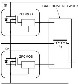
Figure 41. Typical ZPCMOS Drive
