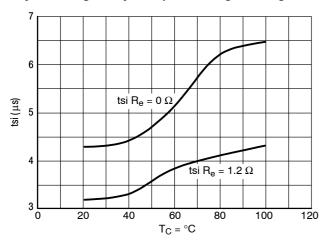
Figure 36.  $t_{si} = f(T_C)$  at  $I_C = Constant$
