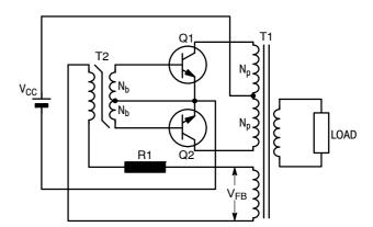
Figure 7. Basic Two Transformer Circuit
