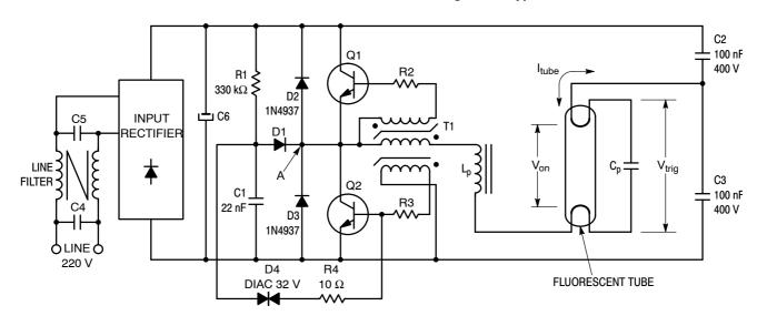
Figure 11. Typical Half Bridge Topology
