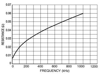
NOTE: Wire is solid copper, one meter long, diameter 2.00 mm, temperature is  $+20^{\circ}\text{C}$ .
