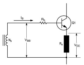
Figure 19. (a) Typical Current Mode Drive
