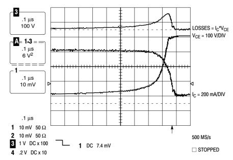
Figure 27. Switching Losses
