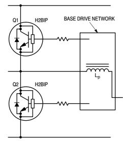
Figure 37. Typical H2BIP Application Circuit
