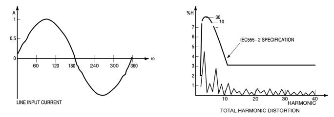
Figure 24. Typical THD of the Evaluation Board
