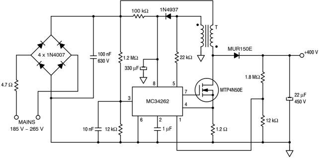
Figure 23. Typical PFC Circuit
