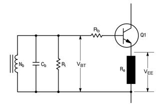
Figure 19.(b) Typical Voltage Mode Drive Circuit
