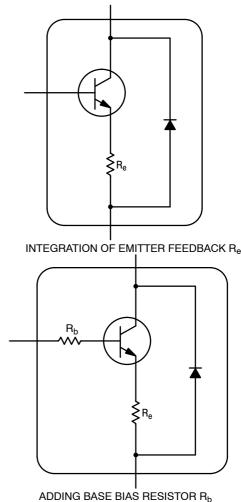
Figure 38. Bias Resistor Integration
