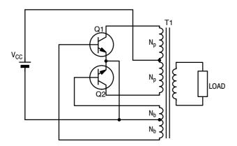
Figure 6. Basic Single Transformer Circuit
