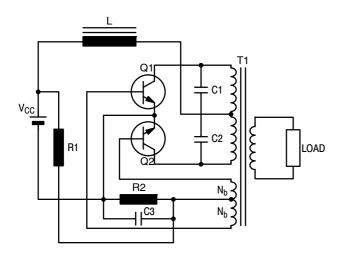
Figure 9. Typical Current Fed, Sinusoidal Output Converter
