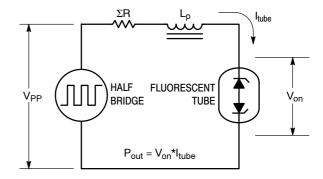
Figure 13. Basic Equivalent Circuit in Steady-State
