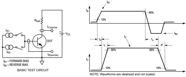
Figure 50. Switching Time Definition
