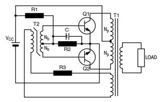
Figure 8. Basic Starting Circuit
