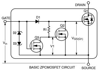
Figure 40. Basic ZPCMOS Internal Circuit
