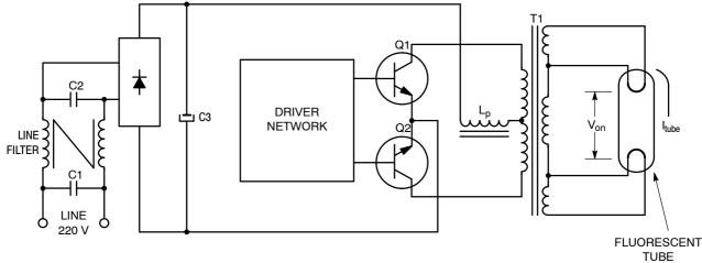
Figure 5. Typical Current Fed, Push-Pull Converter
