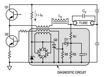
Figure 21. Fault Memorization
