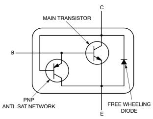
Figure 34. (a) Basic H2BIP Internal Circuit
