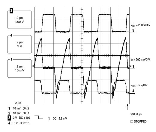
Figure 33. . Drain Current and Gate Voltage in Steady State at  $P_{out}$  =  $P_{min}$
