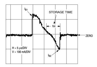
Figure 15. Typical Base Current Waveform
