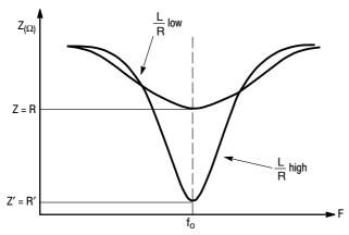
Figure 12. Typical R/L/C Series Network Behavior
