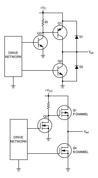
Figure 43. Compound Output Basic Circuits
