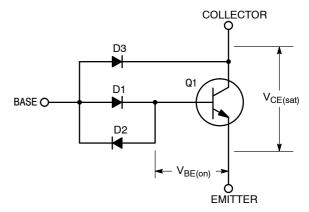
Figure 30. Typical Baker Clamp Circuit
