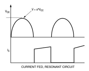
Figure 10. Typical Push-Pull Waveforms
